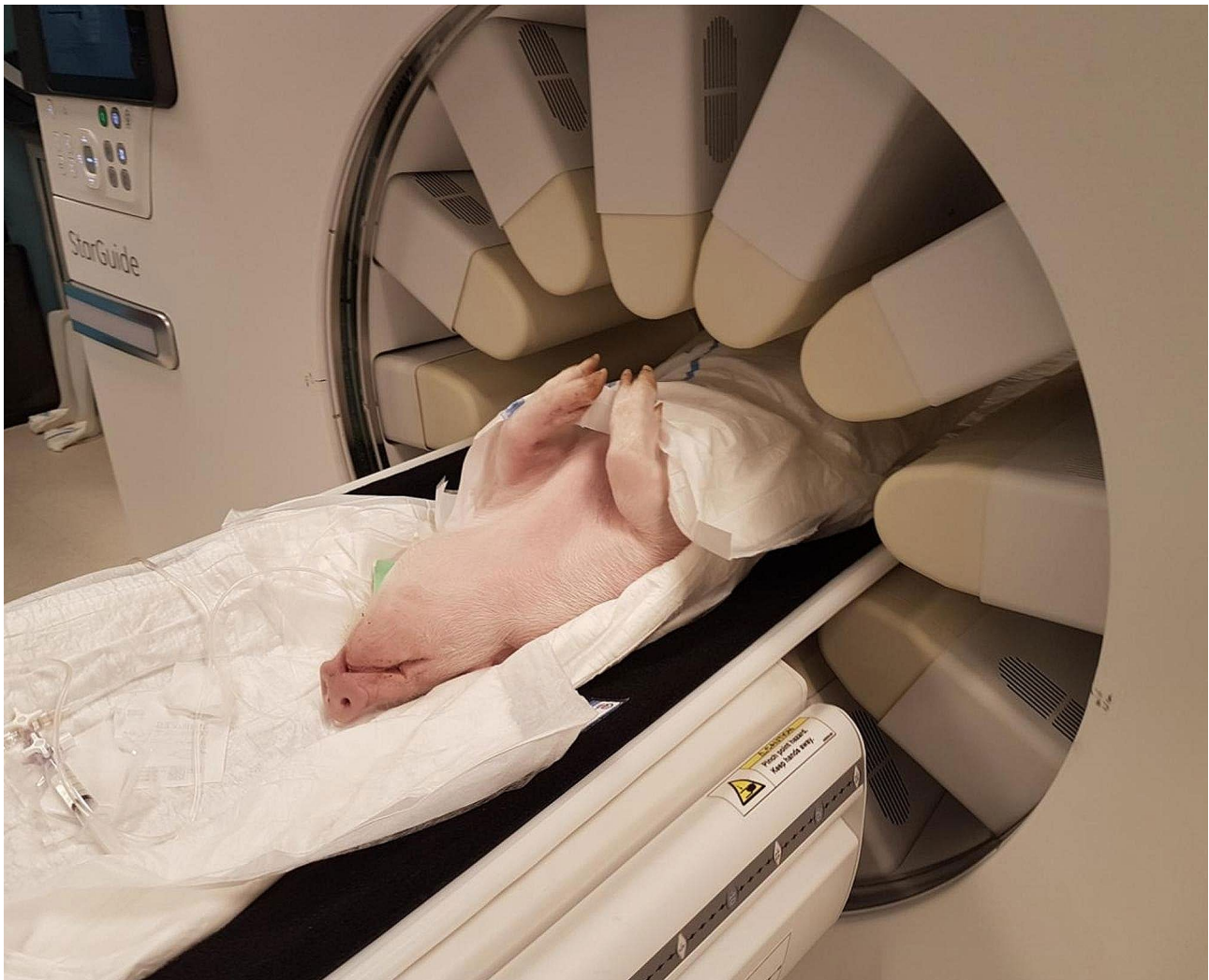
Fig. 1 Picture of the pig during the dynamic SPECT acquisition with the Starguide camera, illustrating the static radial and angular positions of the 12 detectors during the scan
